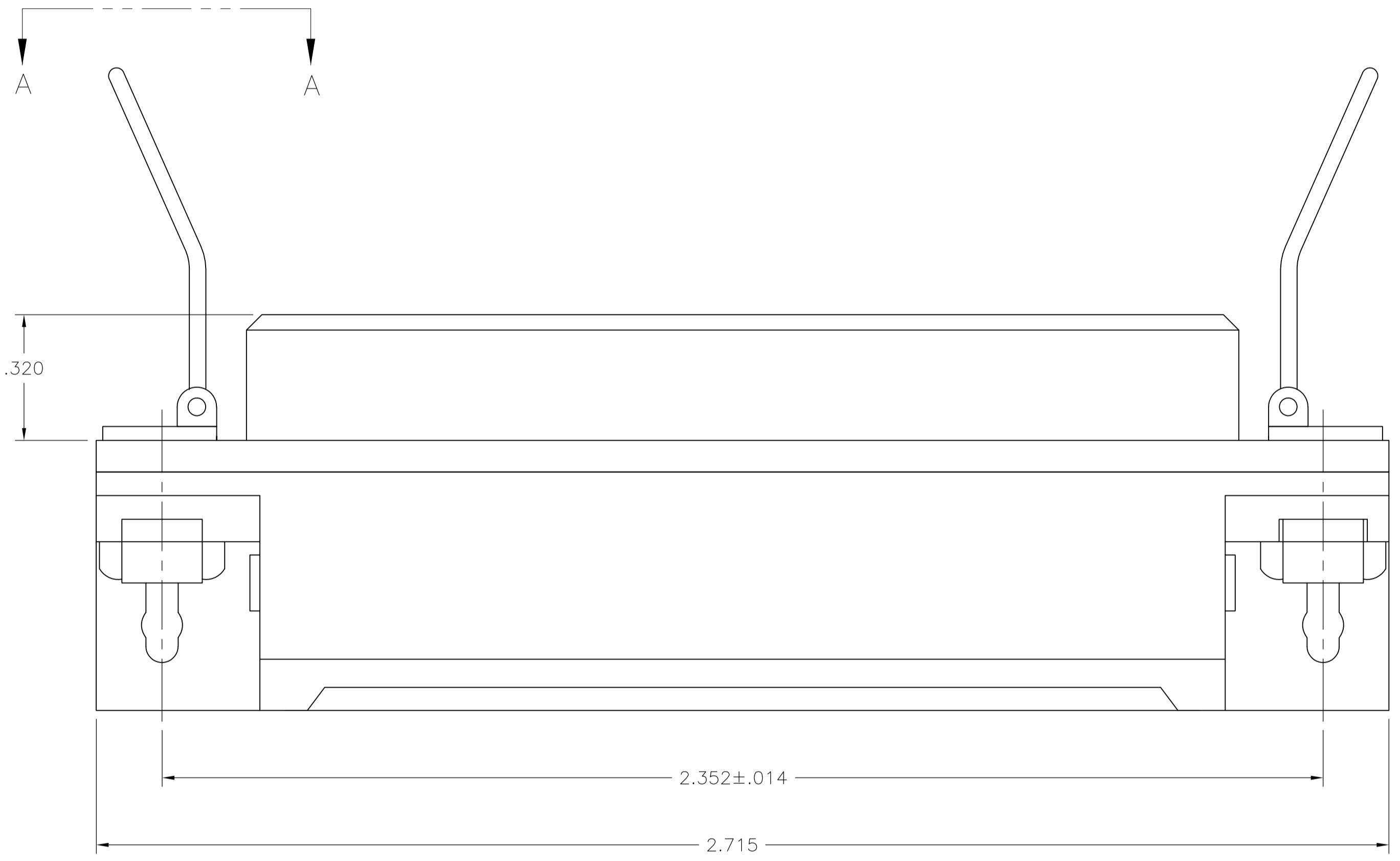
SUGGESTED PRINTED CIRCUIT BOARD MOUNTING DIMENSIONS
